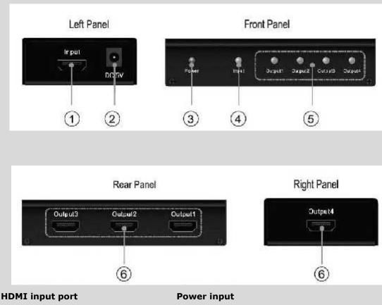
Port indicator of power input Indicator of HDMI output
